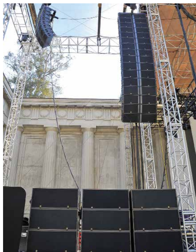
"We brought in an L-Acoustics rig for the two nights at the Greek Theatre in Berkeley," says systems engineer Grabe. "The L/R arrays consists of 16 K2 per side supplemented by eight Kara per side as out-fills and six ARCS Wide as front-fills. The nine SB28s per side are increasingly delayed to widen the coverage."
