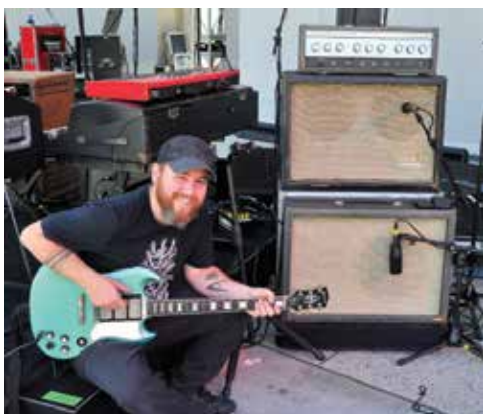
Guitar tech Andy Jones says that Brittany's guitar amps, Sears 1484 2x12-inch and 1x15-inch, are miked with a Beyerdynamic M88 and an Audio-Technica 4040, while guitarist Heath Fogg uses an AEA N22 ribbon mic and Shure SM57 on his amp.
