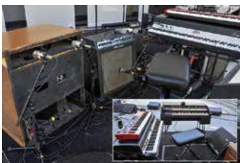
Keyboardist Ben Tanner's mic setup consists of two EV RE 38s on his Leslie top with an ATM 23HE on bottom. The microphone on the Ampeg Gemini 5 is a Telefunken M80, which was chosen for its warmth and expressive midrange.
